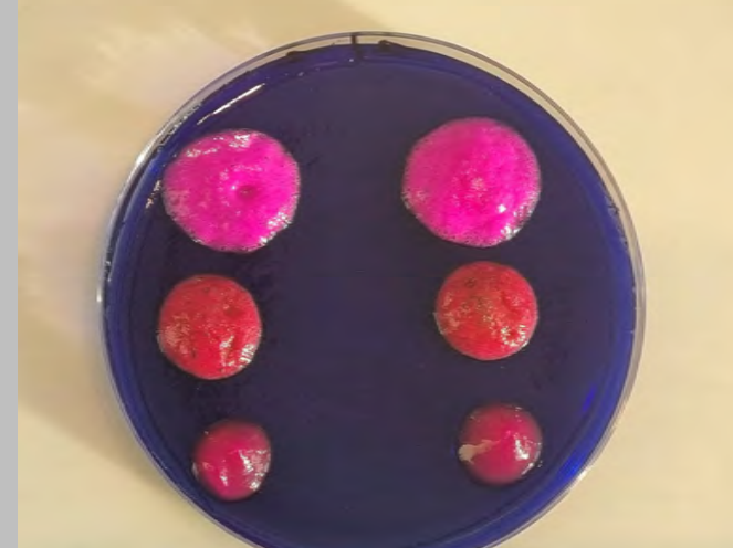
Up: SB gel with gold nano's, middle with NW nano's, down without nano's, 12% H 2 O 2 . Left: no illumination, right 30'' KTP laser, SB protocol, 30' overall interaction time.
