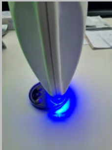
Philips led, induces an overall increase in the in-vitro gel temperature of aproximately 8° C, 3LT, an average of 5° C.
