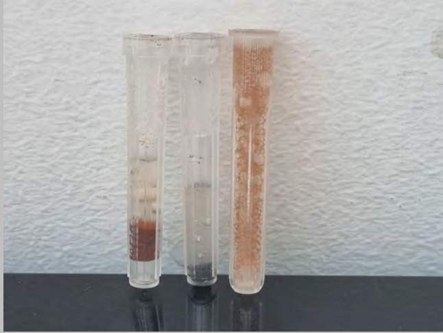
left: nano 1 with 12% H 2 O 2 , moderate reaction. Middle: nano 2 with 12% H 2 O 2 , no reaction. Right: combination of nano 1 and nano 2, severe reaction.
