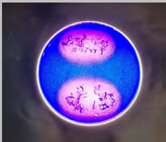
NanoWhite 12% H2O2, 36' interaction time. Up: removing gel, rinsing & drying after 9' and after 18', down: no removing of the gel, both, no illumination.
