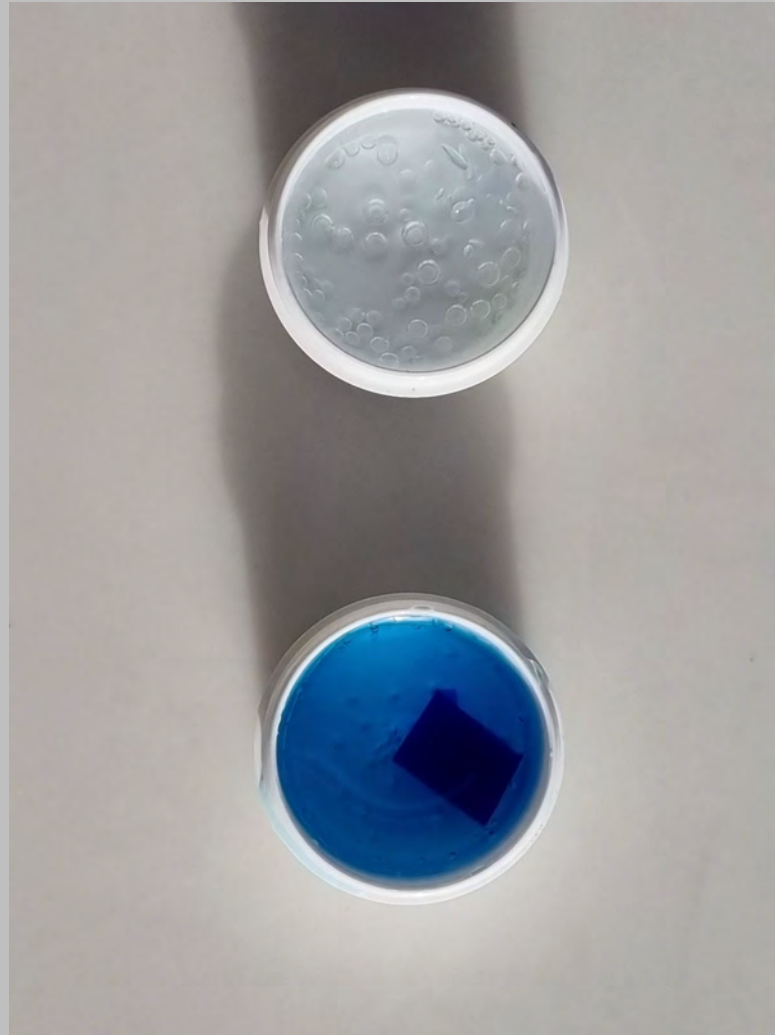
Up, 12% H 2 O 2 , Werken met Merken, down, 30% H 2 O 2 , pharmacy, with a sample of agar-plate-MB. Up, complete oxidation of both MB and agar-gel. Down, even no oxidation of the dissolved MB.
